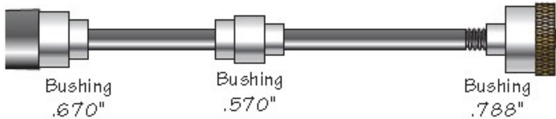
2. Advance a 60° revolving cone center into the dimpled end of the mandrel and tighten using light pressure. **Do Not** over tighten the tailstock or mandrel nut as this may cause the mandrel to flex resulting in off-center barrels.
